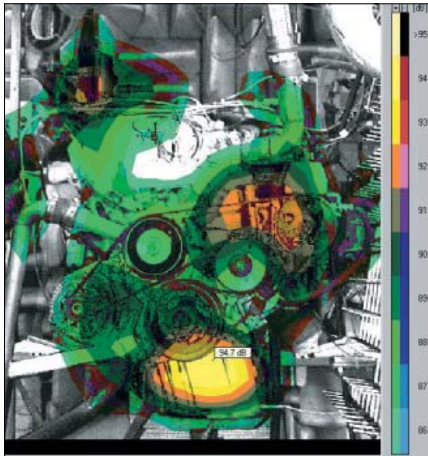
Fig. 8 Average Sound Intensity at the engine surface for the 1 kHz 1/3-octave band. The contour interval is 1 dB
